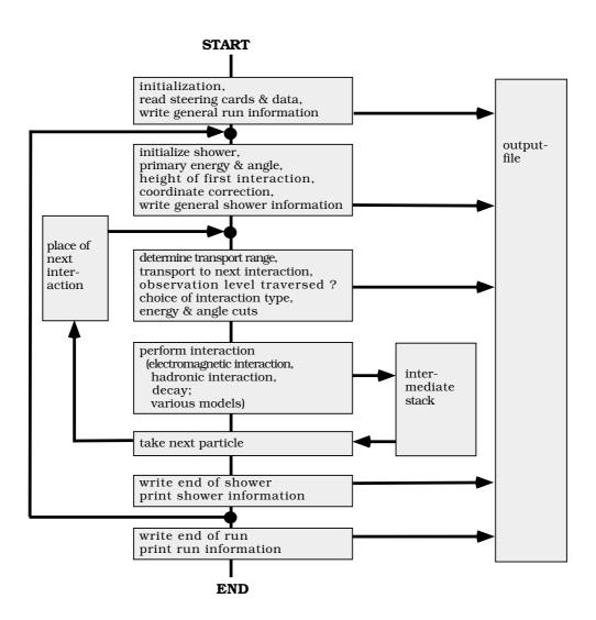
Figure 2: Simplified flow diagram of CORSIKA.
