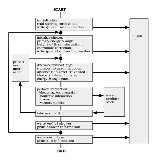
Figure 2: Simplified flow diagram of CORSIKA.
