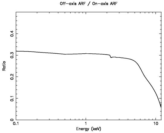
we show the ratio of an off-axis (aprox. 10 arcmin) vs. on-axis ARF values with respect to the energy. The ratio remains almost constant up to 4 keV.
