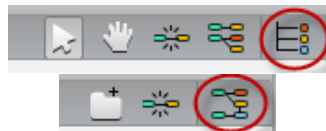
Figure 11.58: 1: Switch to the Project Tree View - 2: Go back to the Project Graph View
