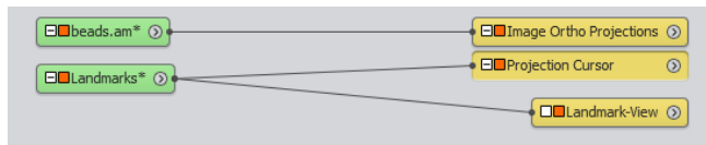
Figure 3.48: Individual beads can be interactively identified using a Projection Cursor module.
