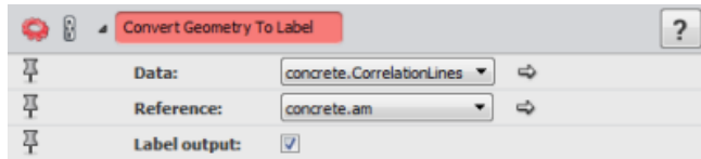
Figure 10.16: Default Parameter Settings of the Convert Geometry To Label Module
