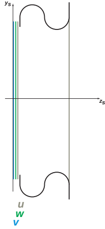
Figure 10.6: The carbon-fibre station body is indicated by the heavy solid black lines. The three doublet layers are indicated by the solid grey ( u ), green ( w ) and blue ( v ) lines. The station reference surface is shown by the solid vertical line coincident with the reference surface of the doublet layer labelled v . The direction y_s axis, defined to be coincident with the v axis and the z_s axes are shown as the solid, black arrows. The x_s axis completes a right-handed coordinate system and therefore points into the page.
